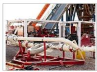
Traditional clamp-on ultrasonic flow meters are typically not used in this application due to their inability to deal with high solids content or entrained gas, and inability to measure through the thick pipe walls generally employed in drilling operations. Additionally, traditional clamp-on ultrasonic meters are not engineered and manufactured for the harsh operating environments typically found on drilling rigs.
