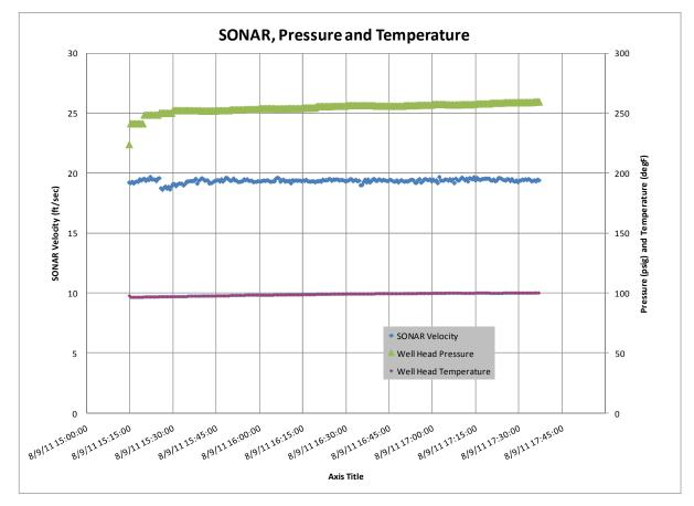
Figure 15: Pressure, Temperature, and SONAR Flow Velocity for 3 hour Well Test on Black Oil Well
