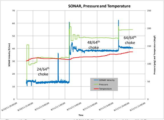
Figure 18: Pressure, Temperature, and SONAR Flow Velocity for 3 Hour Well Test
