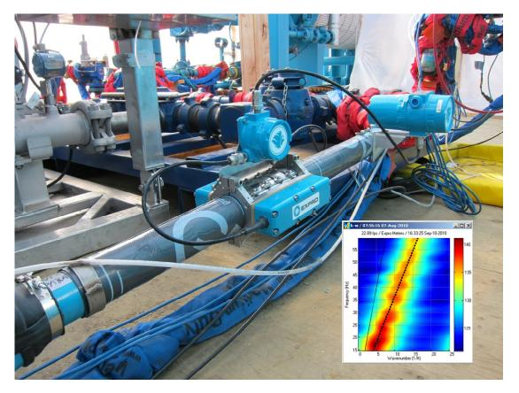
Figure 11: SONAR flow meter clamped-on to a 3-inch, schedule 160 temporary piping on a well test package, downstream of the production choke and upstream of the test separator during Well Clean-up
