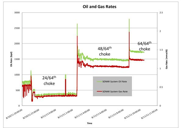
Figure 19: Gas and Oil Rates Reported By TPS1000 Compared to Gas and Oil Rates from Well Test Separator for 3 hour Well Test on ZFOD well ZB3
