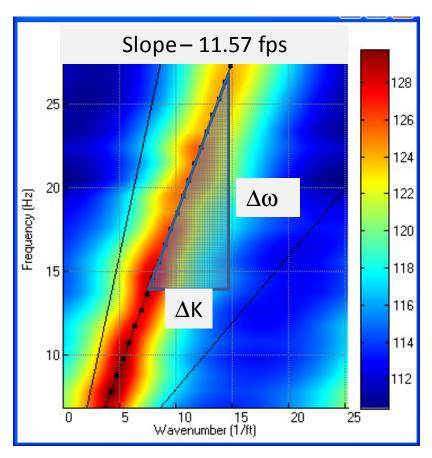
Figure 4: K-w plot from a Clamp-on, SONAR meter on Gas Well
