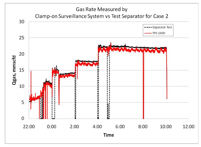
Figure 12: Comparison of Gas rates reported from TPS1000 System and Gas rates from a Reference Test Separator During Well Clean-up
