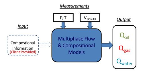
Figure 5: Schematic of TPS1000 Total Production Surveillance Methodology
