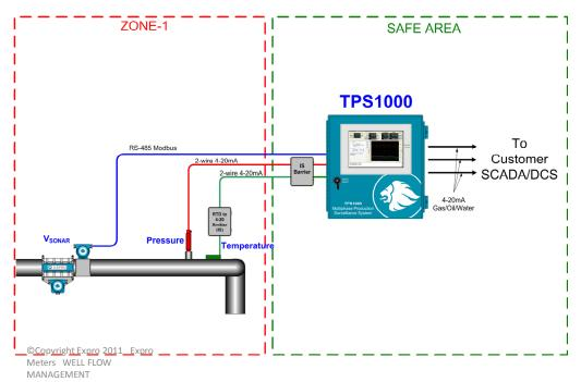
Figure 6: Schematic of TPS1000 Installation
