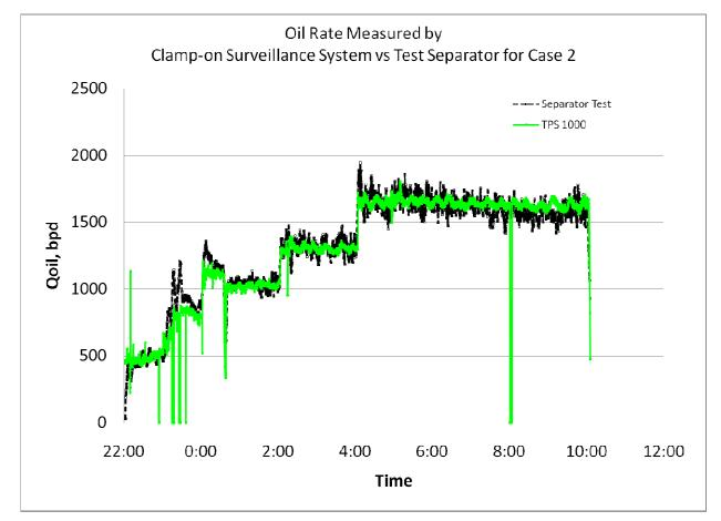
Figure 13 Comparison of Oil rates reported from TPS1000 System and Oil rates from a Reference Test Separator During Well Clean-up
